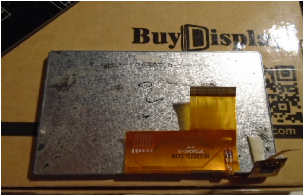
TFT screen on the side of connections to the printed circuit
