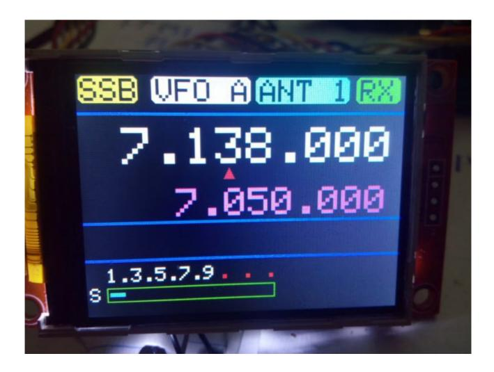
Super-Vfo is really a DDS VFO software program for Arduino Uno and Arduino Pro Mini 16Mhz, with TFT screen 2.2" SPI of 320\*240 (ILI9340 type), a DDS module with AD9850 or AD9851 and one rotary encoder, which it allows all functions of VFO without requiring any button more. It is very easy to use.
