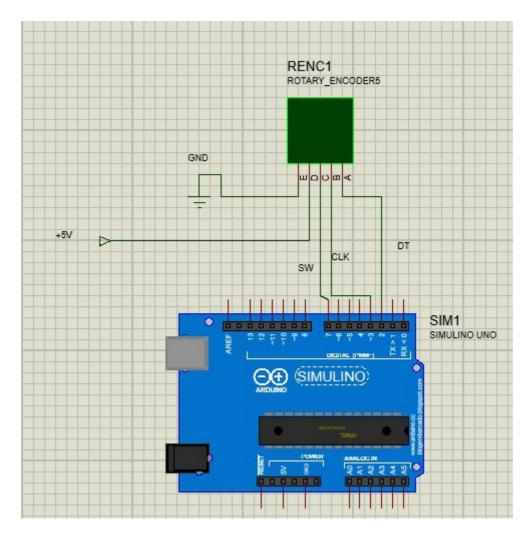
Pin of rotary encoder :GND, +, SW, DT y CLK. Between pin DT and CLK of rotary encoder and GND you must solder a 100nF Capacitor respectively to minimize rebounds of rotary encoder. Pin DT of rotary encoder connected to Pin 2 of Arduino.Pin CLK of rotary encoder connected to Pin 3 of Arduino. Pin SW of rotary encoder to Pin 7 of Arduino.Pin GND of rotary encoder to GND of all VFO.
