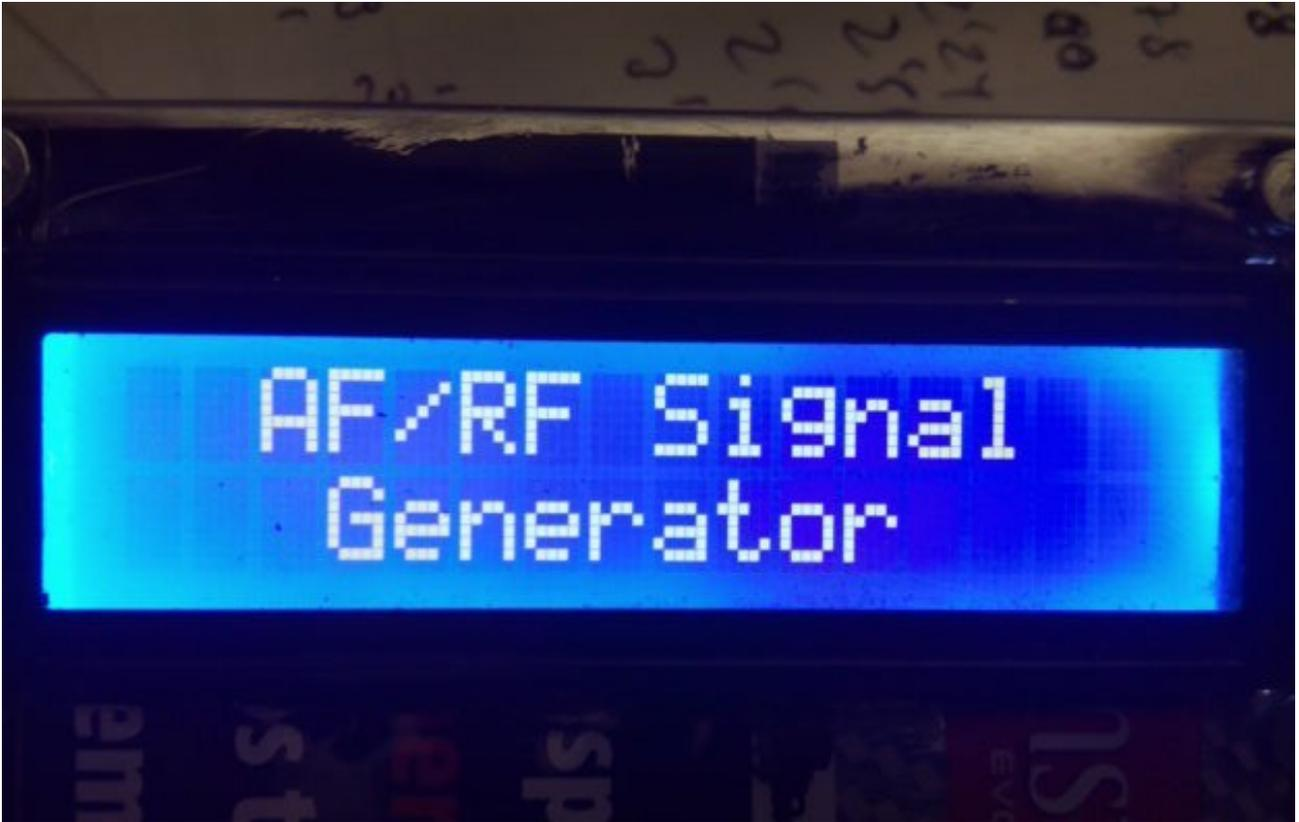
AF/RF Signal generator is a simple and useful circuit create to Arduino Uno or Arduino Pro Mini 16Mhz, with a LCD de 16X2 with I2C interface, a DDS with AD9850 or AD9851 chip ,a set of 8 attenuators and one rotary encoder that allows all the operation .Range operation is between 20Hz to 32Khz for AF mode and between 100Khz to 40 or 71 Mhz according to DDS used in RF mode.
