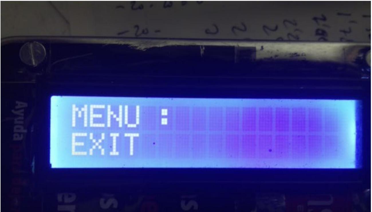
The first function is **EXIT**. If you press again the button encoder you return to normal mode of operation of Signal Generator. If you turn the encoder you access to next option.
