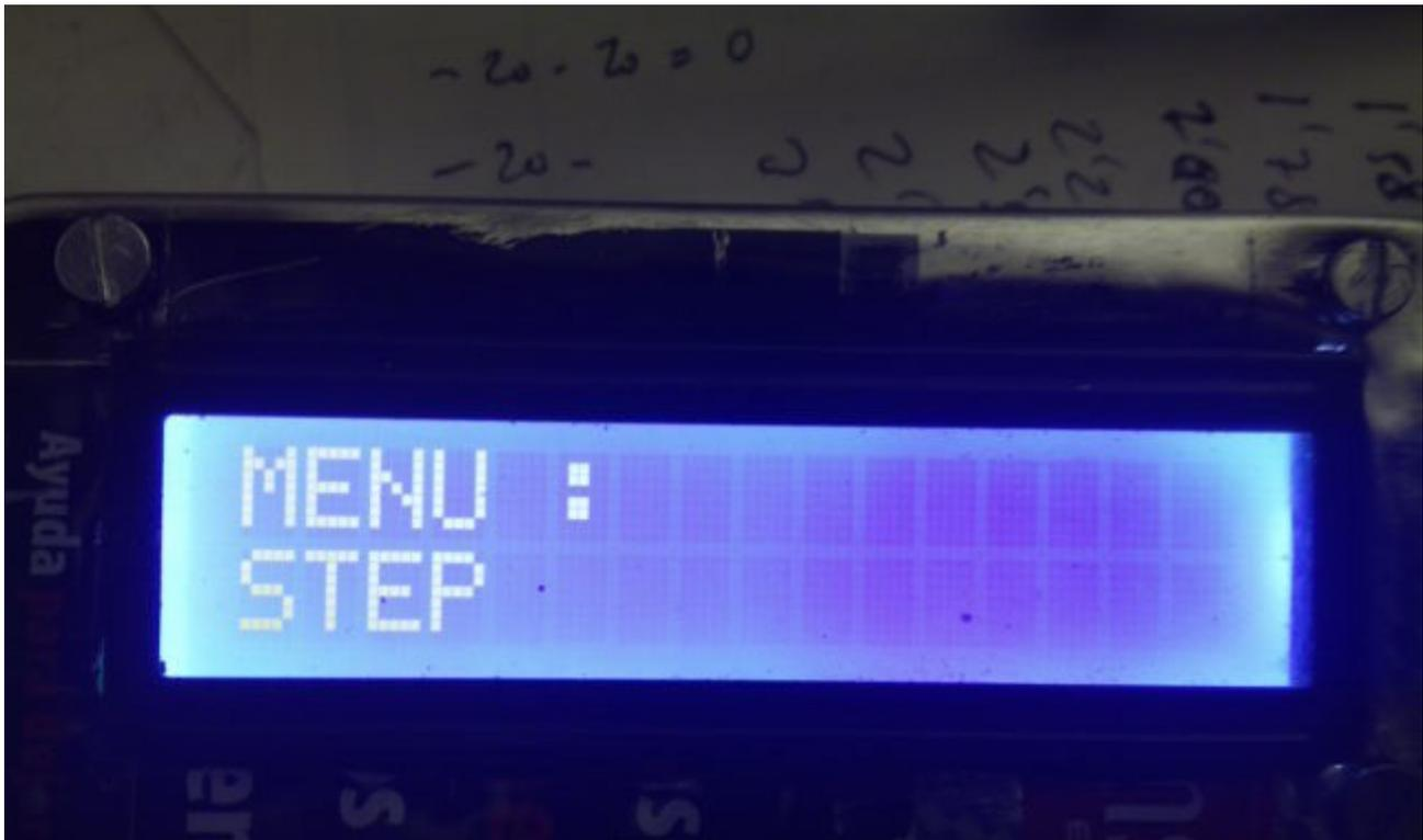
**STEP** , you can changed the step of frequency. Default value are 1 Hz. Press button encoder to select step. Turn encoder you can select the step. Values are: 1Hz,10Hz,100Hz,1Khz,10Khz,100Khz and 1Mhz. To save this value press again encoder button. You can select diferent step for AF or RF mode.
